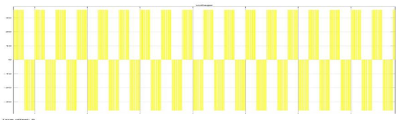
Figure 3. Voltage wave form of 3-Level NPC.
